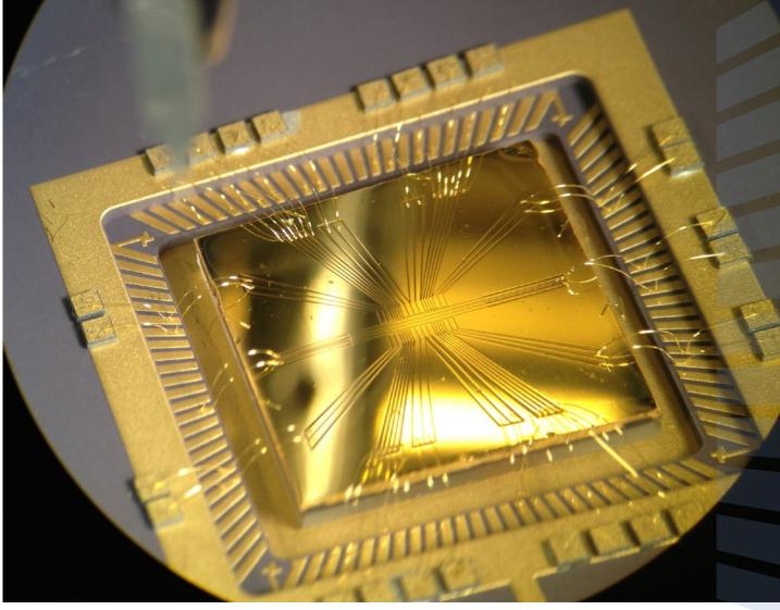
An ion trap from the Oxford University Ion Trap Group. The ions are held in vacuum just above the surface using electric fields / D. Aude-Craik & D. Allcock
