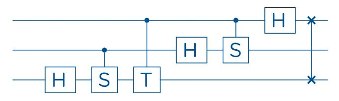
Figure 2: A subroutine of a quantum Fourier transform algorithm, to be read from left to right. Each row is a single qubit. Squares with H represent a single-qubit rotations called Hadamard. Vertical lines represent two-qubit gates.
